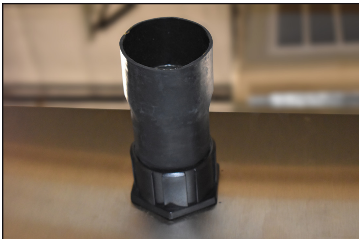
Figure 6 – VJT entry port and RTD connection point
