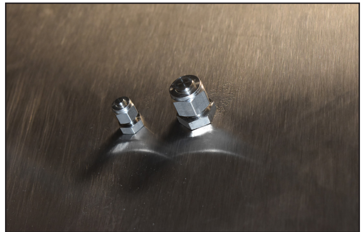
Figure 5 – Ports for Accumulator Tank Burst Disk and Relief Valve
